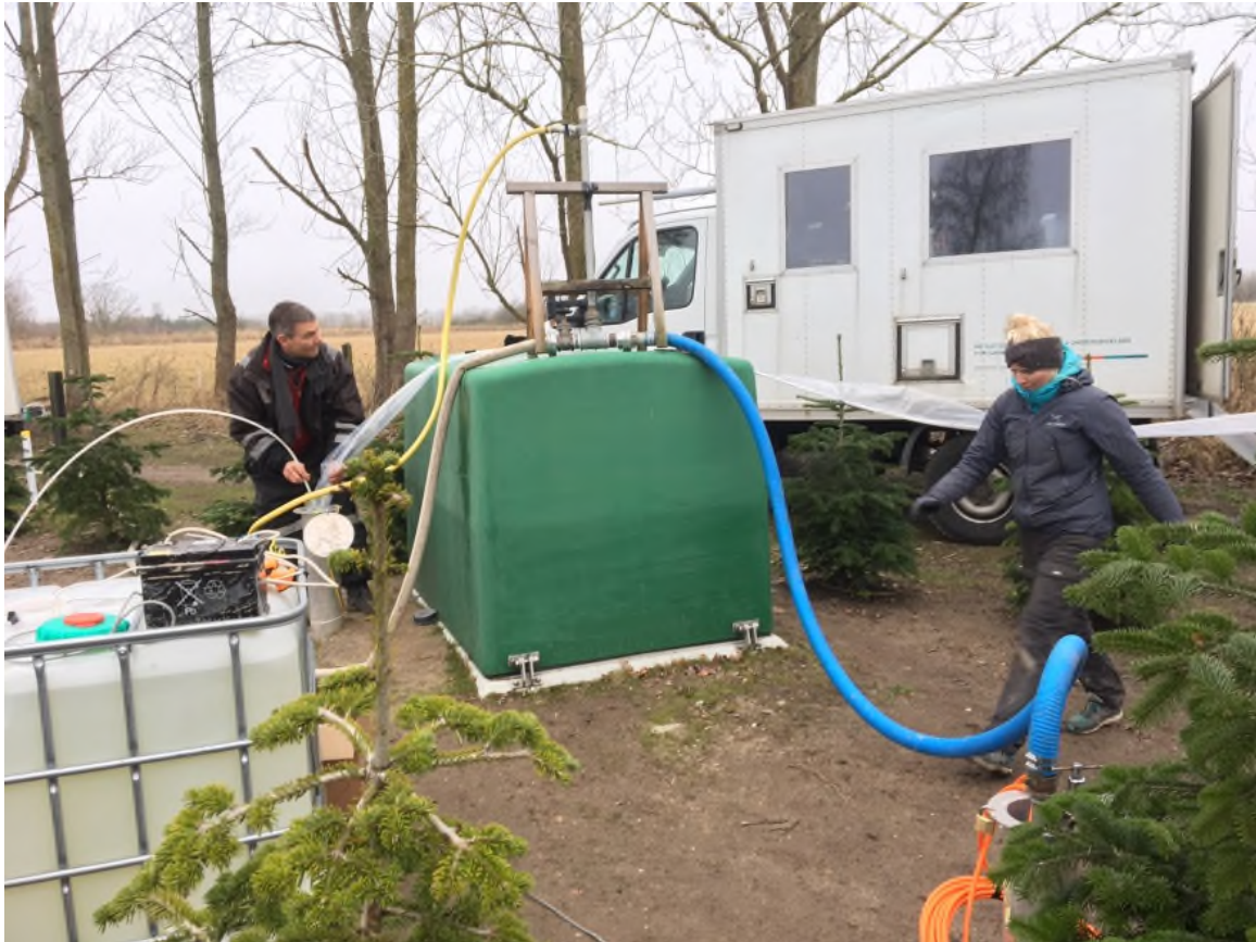
Figure 15. Injection of tracer into T1 just left of the green cover, through thin white hose – about 1 meter from the WSP no. 9 below the green cover. Blue hose injects water pumped from UB2 into UB1 to create the dipole flow field between UB1 and 2 Illustrated in Figure 14. The manifold on top of the green cover is for removing air from the water prior to injecting it. The transparent plastic tube going into T1 was filled with water after the tracer injection to expel the volume of water in the well to avoid effects of the borehole during the tracer movement.
